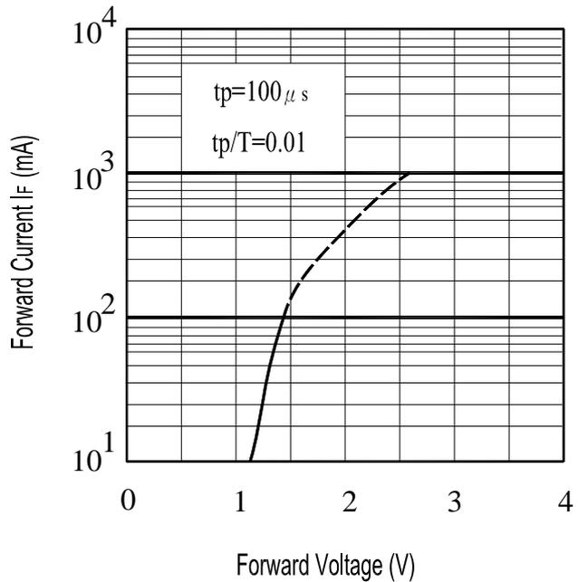
**Typical Electro-Optical Characteristics Curves**
